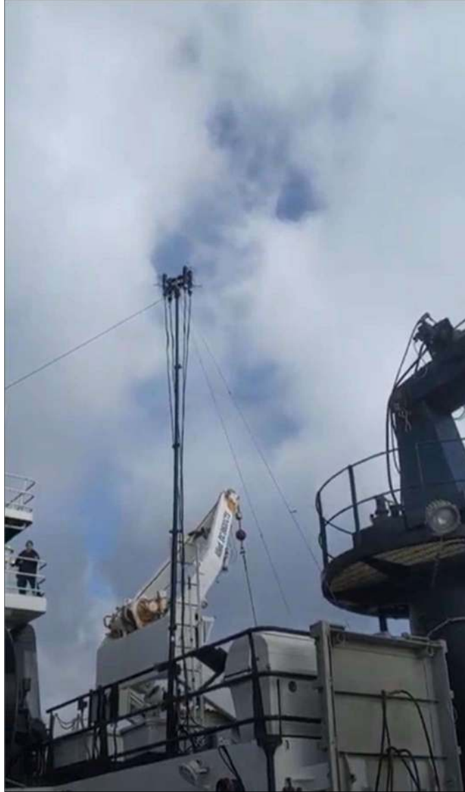
Figure 8. E_s sensors mounted atop of telescoping pole at the upper structure of NOAA Ship Bell M. Shimada .
