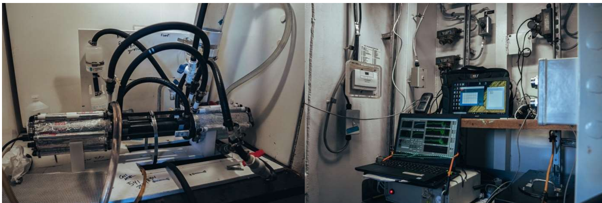
Figure 31. (Left) An inline system with the AC-S, filters, and tubing, including an aluminum jacket to keep the AC-S at a similar temperature to the water it was measuring, limiting any condensation on the inside of the optical windows. (Right) Computer setup with the logging software used and the light trap for the BB3 in the bottom right corner.
