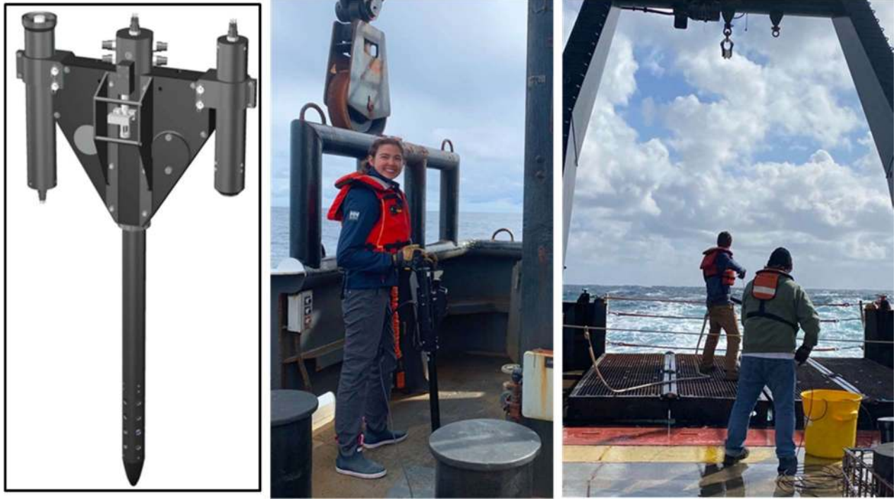
Figure 24. Left is a constructed image of the HyperPro-II profiler system, consisting of the dart and wings (body) connected to two hyperspectral radiometers. Middle is a picture of the HyperPro-II being transported by Wave Moretto from the deck to the fantail for deployment. Right is the deployment of the HyperPro-II off the fantail.
