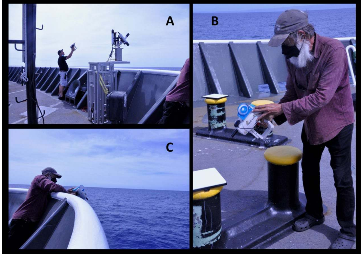
Figure 9. Illustration of the station collection sequence for above-water R_{rs} . (A) Sherwin Ladner (NRL) was collecting the sky measurement sequence. (B) Charles Kovach (NOAA) was collecting the white reference plaque sequence, and (C) Charles Kovach (NOAA) was collecting the water sequence. The above-water spectroradiometer shown in all images is the ASD with an inclinometer attached to maintain the desired measurement angle of 40^\circ .
