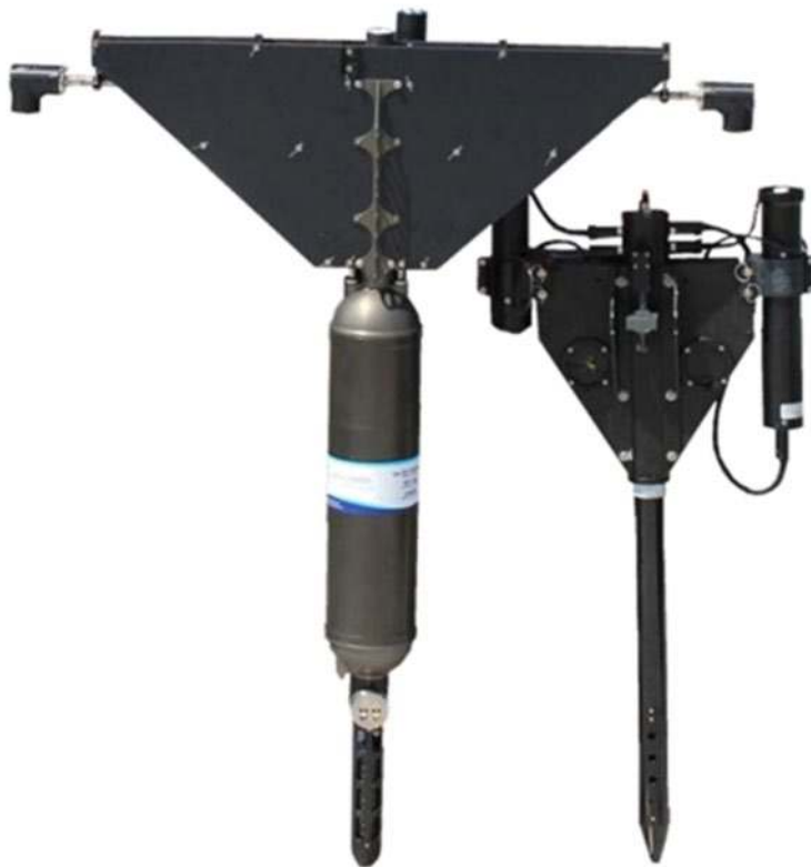
Figure 27. Comparison of HyperNAV (left) and HyperPro-II (right)
